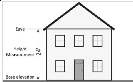
Figure 22-1: Where to Measure Eave Height
